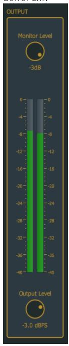
Adjust the Output Level to set the gain feeding the stream encoder. Changes made to this knob will be reflected in the metering. As with the input, this meter displays peak, not average and levels should hit between -12 and 0 without exceeding 0. The default level set to -3
