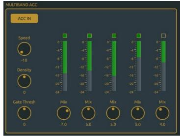
Located directly above each gain reduction meter is the GATE indica- tor for the band. The GATE indicator will be ON (lit) when the input level to a band is *above* the setting of the Gate Thresh control. In other words, a lighted Gate indicator shows that a band is actively engaged.
