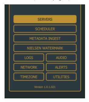
If your unit doesn't already appear in the Server box, in the Add New box, type the IP address for the WAN or LAN port of your WheatStream device and click Add. You will automatically connect.
